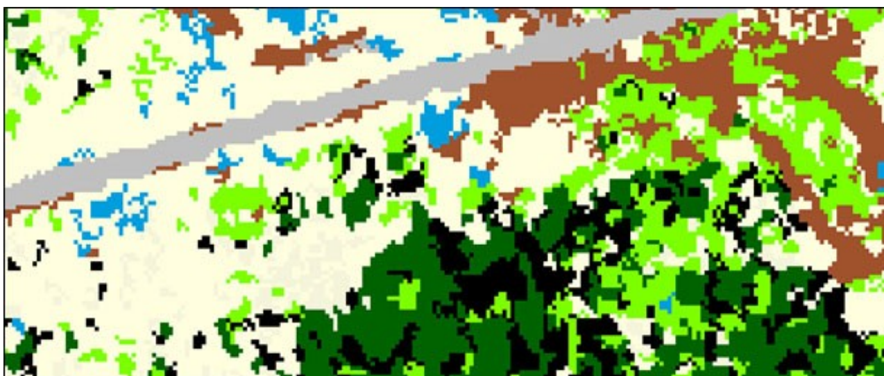
Figure 11: Supervised maximum likelihood classification of the World View 2 image. Legend: grey = road, blue = water body, cream = barren land, black = shadow, brown = shrub, bright green = climber, dark green = forest.
