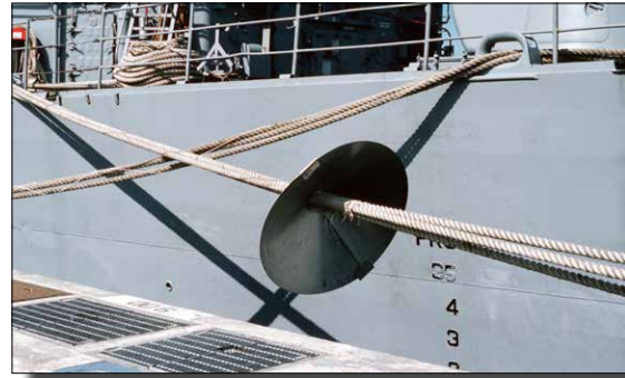
A rat guard mounted on the mooring line of a United States warship. Photo: U.S. National Archives.
